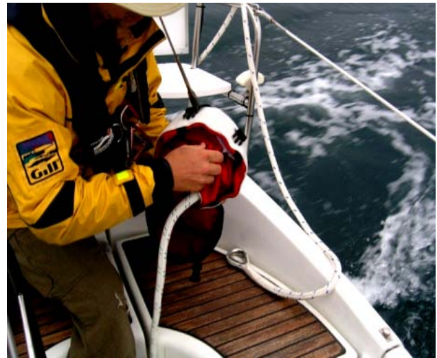
Allow the 10-foot (3 m) "drogue tail" to fall out of the Para-Ring.
