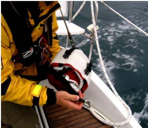
Squeeze the mid section of the two vinyl buckles to open the bottom lid.
